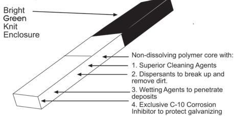
The green knit enclosure lets water pass through to contact all of the surfaces.
